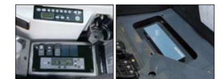
Air conditioner / AM-FM radio (Cab) Tool box (canopy)
